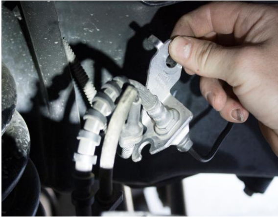
Figure 3A: Passenger ABS Line Removal
