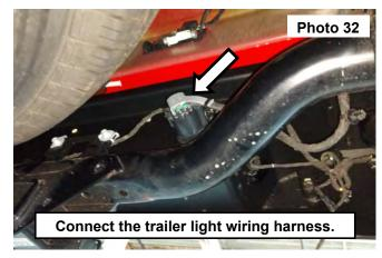
34. Connect the wiring harnesses from the bumper to the vehicle. Secure any wires from hanging or any heat source. See Photos 33 and 34.
