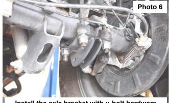
Install the axle bracket with u-bolt hardware
