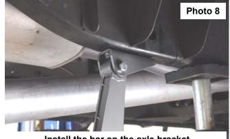
Install the bar on the axle bracket
