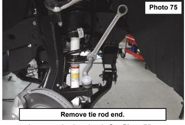
80. Place the tie rod end into the knuckle to hold it, using a 24mm wrench, remove the tie rod end. See Photo 75.
