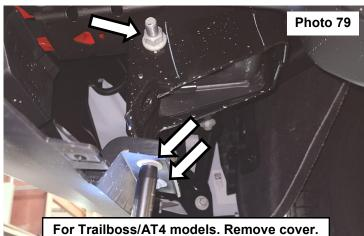
Plug in rack and pinion and diff actuator.
