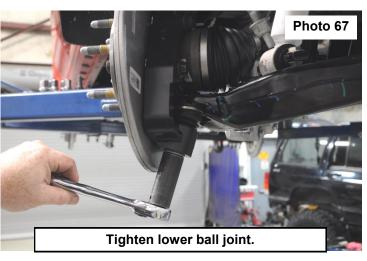
bearing. Torque using a 24mm socket to 40ft/lbs + 90°. See Photo 67.
