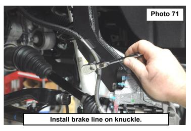
78. **2019 Models skip to next step.** Install the supplied brake line relocation brackets (217BAG6) on to the knuckle using the factory hardware. Tighten using a 10mm socket. Attach the factory brake line bracket to the new supplied bracket using the supplied 1/4" x 3/4" bolt and nut (217BAG6). Tighten using a 7/16" socket and wrench. **See Photos**
