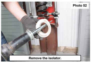
57. Remove the factory lower coil spring isolator from the OEM strut. See Photo 52. Save for reuse.
