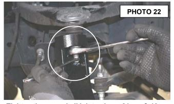
Tighten the upper ball joint using a 21mm & 10mm.
