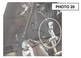
Install bracket to secure the brake line.
