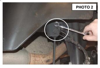
4. Remove sway-bar link using 8mm and 18mm wrench for lower end and 18mm for top end. See Photo 3 & 4.
