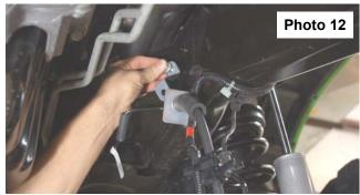
5/16" x 3/4" bolts, washer, and nuts. Tighten with a 13mm socket and wrench.
