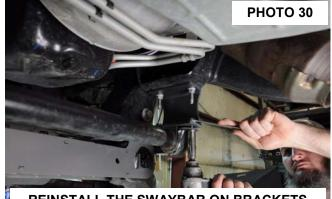
**REINSTALL THE SWAYBAR ON BRACKETS**
