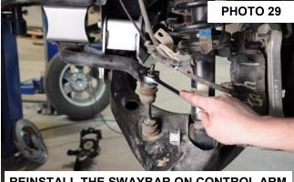
**REINSTALL THE SWAYBAR ON CONTROL ARM**
