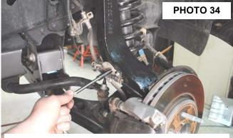
**INSTALL THE BRACKET TO KNUCKLE**
