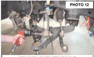
**REMOVE LOWER STRUT BOLT**
