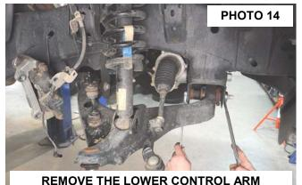
18. Remove the strut from the upper mount using a 15mm socket / wrench. Retain hardware for reuse. **See Photo 15.** 19. Remove the bearing from the stock knuckle with a 18mm socket. **See Photo 16.**
