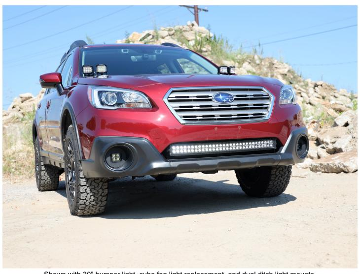
Shown with 30" bumper light, cube fog light replacement, and dual ditch light mounts.
