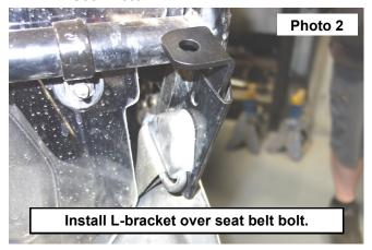
Install the supplied 3/8"-16x1" bolts, nuts, and washers above the stock hardware using a 9/16" socket/wrench.
