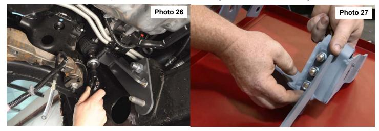
32. Install upper control arm drops onto truck using supplied 9/16" x 4" bolts and nuts using four cam lock washer per side with one cam lock washer with a tail on the back side for the ABS wire. **See Photo 29.**
