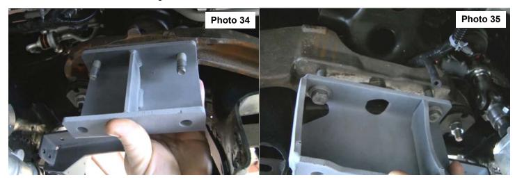
37. Install diff using new supplied 12mm x 45mm bolts and nuts. Be sure not to hit or push diff into rack and pinion. Use new bolts and nut on driver side and use new bolts with old stock nut on passenger side. Use a 18mm and 19mm socket and wrench for new bolts and a 21mm for the stock nuts. Plug in the 4x4 actuator and vent tube. See Photo 36.
