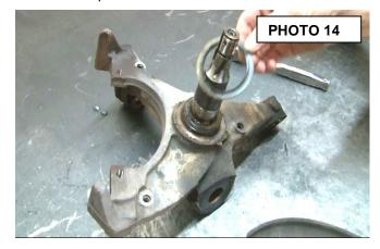
18. Place dust shield on new spindle using stock hardware. Tighten with 13mm socket. See Photos 16 & 17.
