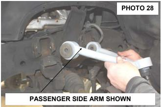
41. Install the control arm on the stock knuckle with factory nut and supplied cotter pin. Tighten ball joint to 50 ft/lbs with a 18mm wrench. **Do not over tighten the ball joint**. Tighten the control arm to frame hardware using a 21mm wrench to 90 ft/lbs. **See Photo 29.**
