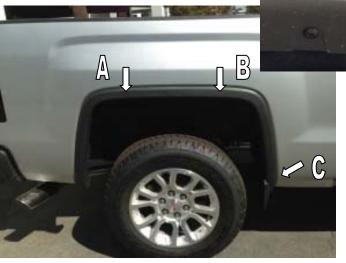
**STEP 12:** Place Fender Flare on the vehicle into the position of best fit. Note where the slots in Fender Flare at positions **A** and **B** align with the existing screws in the vehicle wheel arch molding. Also note where the slot in the Fender Flare aligns with the front mud flap deflector, position **C**. Remove Fender Flare. Remove the existing vehicle screws in location **A** and **B** using #15 Torx head screwdriver. Maintain screws for re-install.
