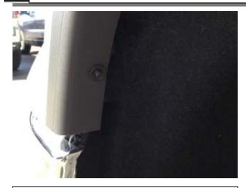
**STEP 7:** Using a 7mm or 8 mm socket, remove upper front wheel arch molding screw. Maintain screws for reinstall.
