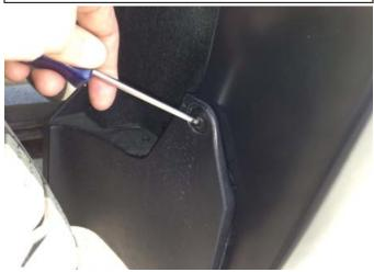
**STEP 14:** Place Fender Flare on the vehicle into the position of best fit, slide the bottom front end of Fender Flare between the existing mud flap deflector and wheel arch molding so that the slot in the Fender Flare is under the vacant hole in the mud flap. Using #15 Torx head screwdriver, loosely re-install the previously removed screw. Ensure the installed rubber seal from STEP 3 is resting firmly on the mud flap deflector.
