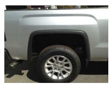
**STEP 11:** Clean the body area where the Fender Flares will make contact. Ensure fenders are dry prior to install.
