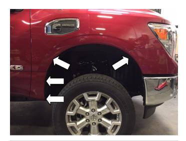
**STEP 5:** Place Fender Flare on the vehicle into the position of best fit. Note where (4) slots in Fender Flare correspond with (4) existing screws in the vehicle wheel arch molding. Remove Fender Flare. Remove the existing vehicle screws in locations as shown with #2 Phillips head screwdriver. Maintain screws for re-install.
