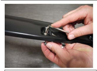
**STEP 1:** Attach the provided bolts and nuts to each Fender Flare using a 3/16" Allen key and a 10mm wrench/socket (wrench /socket and Allen key not supplied). Ensure inside of Fender Flares where the rubber seal is attached is clean, using the alcohol wipes provided. Wipe away any residue with a dry clean cloth.
