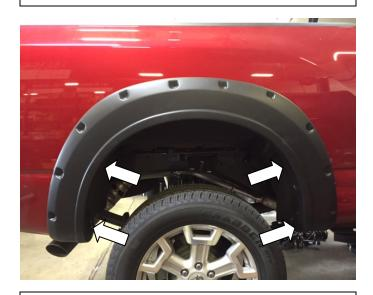
**STEP 10:** Place Fender Flare on the vehicle into the position of best fit. Note where (4) slots in Fender Flare correspond with (4) existing screws in the vehicle wheel arch molding. Remove Fender Flare. Remove only the existing vehicle screws in location as shown with a #2 Phillips head screwdriver. Maintain screws for re-install.
